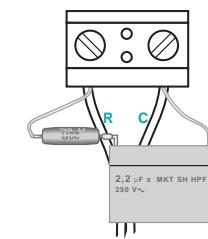
Motor, relay, neon, transformer (max power 1000 VA)
